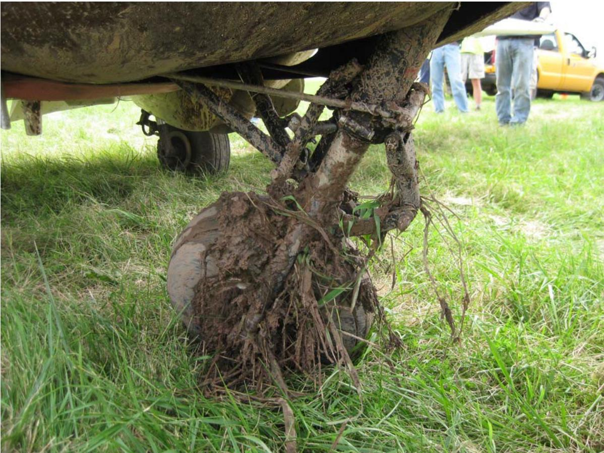
**Bellanca, 1730A, Failed Nose Landing Gear, ATA 3230**
